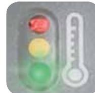
Temperature gauge alerts operator if motor overheats to help prevent unnecessary burnout while blending back-to-back batches
