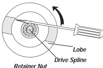
\*For best results we recommend using a Retainer Nut Wrench in place of a screwdriver. To order ask for Item #1222
