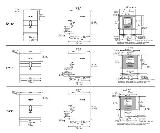
INSTALLATION NOTE: Allow 6" minimum space at sides and back for ventilation and utility connections.
