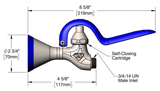
Flow Rate: 1.15 GPM [4.35 Lpm] @ 60 psi [4.14 bar] Spray Force: 7.5 Ozf [212 Gramf] @ 60 psi [4.14 bar]
