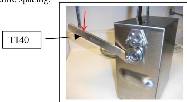
**Caution: Thin spacers washers (W034, W140, W141) are often used to control the gap or spacing between the knife and the gear. Inspect the worn gear when removed to be sure spacer washers are not stuck to the gear. If they are present clean them and return them to the output shaft behind the gear.**
