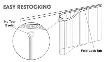
Employees will also appreciate the CASER®. They can restock or clean the coolers quickly and easily. Just fold back the edge and attach the "foldlock" tab and you can quickly replace product.
