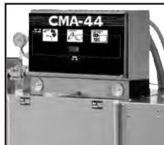
Single action control switch with easy to read temperature gauges and complete operating instructions.
